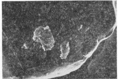
FIG. 6. Carbon replica of a starch grain from a mixture with 0.5 per cent light magnesium oxide showing the fine particles attached to the surface in aggregates \times 6,600 .
